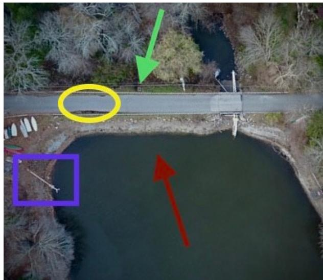
sluice gate location (green arrow), auxiliary overflow spillway (yellow oval), and primary service spillway no longer meet the current State Department of Environmental Conservation (NYSDEC) requirements.
