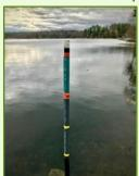
In this Spillway Dam Lake Gauge photo, the teal-colored section represents the summer level range of one foot above the spillway deck when the weir boards are in place. The yellow lines represent the number of feet below the spillway deck (or below the winter level when the weir boards have been removed). The black circle in the water behind and to the left of the teal blue section is the whirlpool that had formed over the west siphon intake, which was the most reliable siphon this year.
