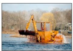
Mechanical Raking: Mechanical raking, also called hydroraking, consists of a specialized paddle wheel propelled barge with a york rake mounted on a backhoe arm. The rake is lowered into the lake sediment, and pulled until full (usually about 0.5 cubic yards). The material is then placed on shore for dewatering, and eventual disposal. Although a slow process, this method does provide multi-year control since most of the plant is removed, not simply cut as
